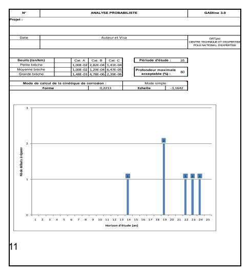
The diagram shows the number of defects for which the failure probability exceeds the criteria, for each year over a period of time
