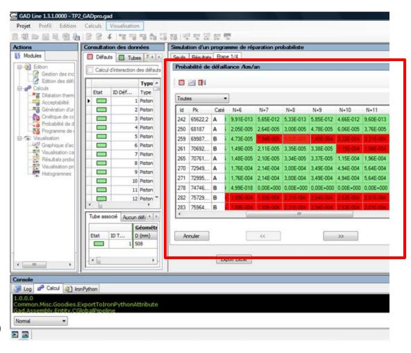
The table shows when the failure probability of a feature exceeds the criteria
